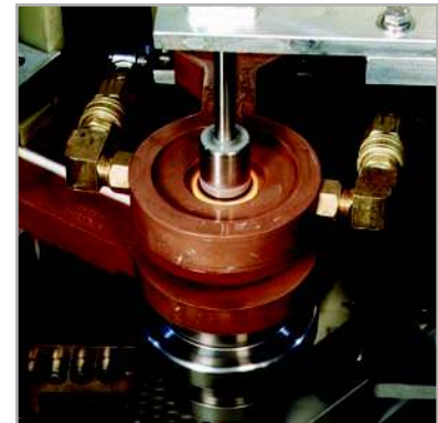
Hardening and tempering a spline
